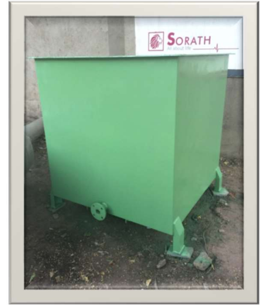
FRP Coated Tank
